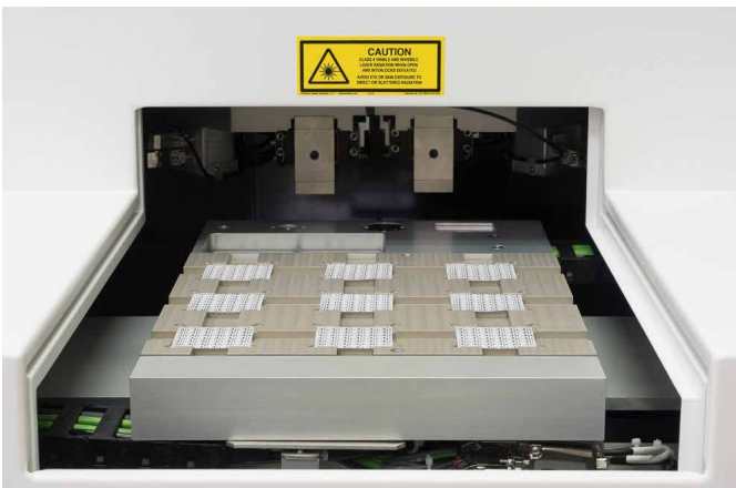
9-up fixture plate for locating 50x50mm substrates. Different fixtures can be exchanged in seconds.
