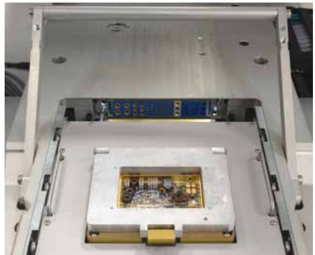
Hybrid package loaded into PPI's universal test fixture with customer-specific test socket for active trimming.
