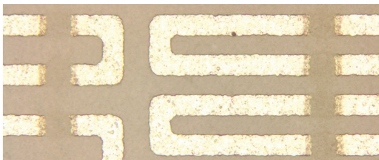
Platinum film links cut with short-pulse laser.
