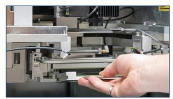
Easy exchange of cable-free chip-R probe cards.
