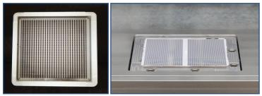
Backlit substrate (L) and temperature-controlled chuck (R).
