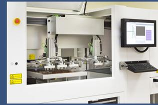
UV laser system, providing high speed processing of copper, and high quality drilling and cutting of dielectric material. ProVia FP-U laser drilling systems are able to machine copper and provide higher process quality in many dielectrics.
