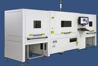
ProVia FP-UC laser drilling and cutting systems incorporate both UV and CO<sub>2</sub> lasers and scan heads. The CO<sub>2</sub> laser is appropriate for high speed drilling, cutting and skiving of dielectrics, while the UV laser is able to machine copper and provide higher process quality in many dielectrics.
